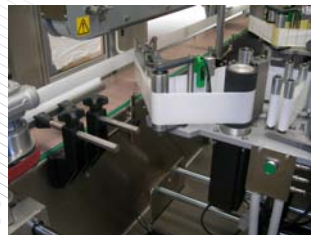
◀ 2 Automatic K320 labeling heads for high speed with SERVO engines.
